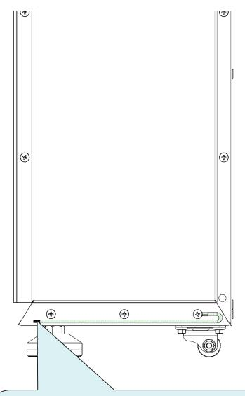
Please use a wire no smaller than 2.5mm<sup>2</sup> to connect the ground wire reserved in the battery pack to the ground wire. This step is crucial for the normal operation and safety of the device, so please make sure to connect accurately.
