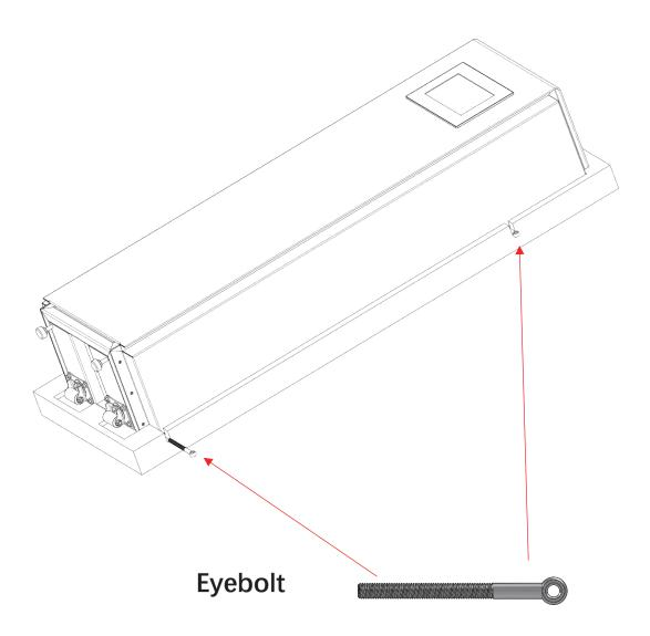
After opening the wooden box, please place the four eyebolts that come with the box into the load-bearing bolt holes at the rear end of both sides of the box. These four eyebolts serve as temporary mobile auxiliary grips or bearing points during lifting operations.
