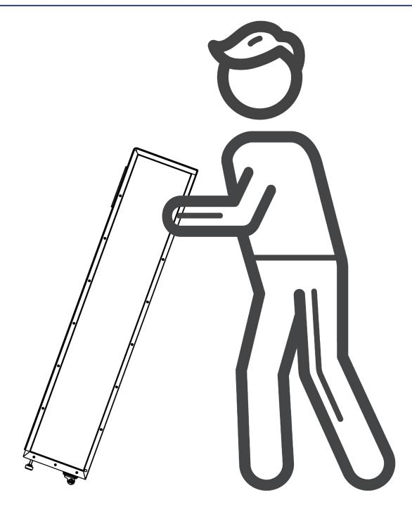
Facing the back of the battery box, hold the eyebolts on the left and right sides of the upper part with your hands, tilt the battery backward about 20 degrees, and use the universal wheels at the bottom of the box to move a short distance. Please do not tilt the battery too much, because the battery is heavy, and if the tilt angle is too large, your hands may not be able to support it, causing the risk of the battery falling.
