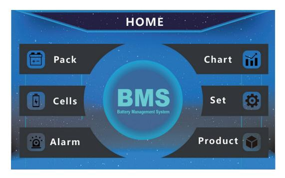
The LCD display shows various critical data, including operating status, real-time including the remaining battery capacity, operating status, real-time power, and fault alarms. Through the LCD display screen, users can clearly see the battery's voltage, current, temperature, and other data. Additionally, it supports touch operations, allowing users to conveniently monitor the battery's status and manage its usage in real-time.
