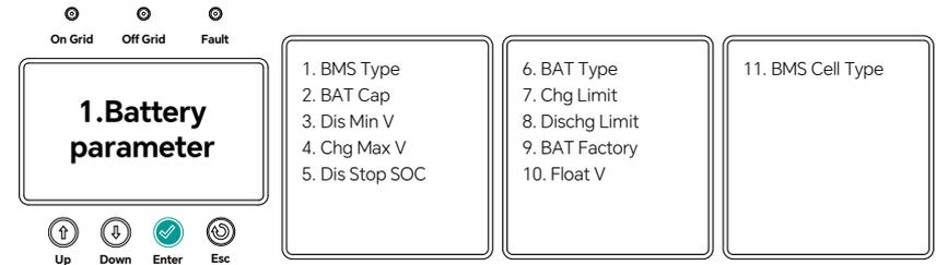
1. BMS Type: Battery charge and discharge maximum current mode (0: default 1: battery control charge maximum charge current; 2: battery control charge and discharge current maximum)
