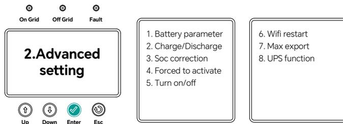
1.Battery parameter Battery parameter setting. This sub-menu screen has 11 options. It is divided into three pages.
