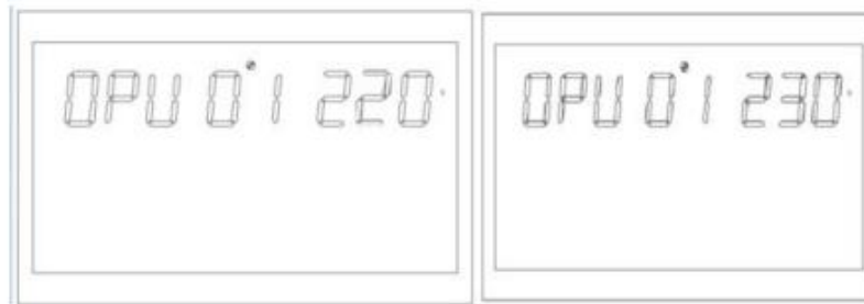
Figure 1-12 Setting the output voltage
