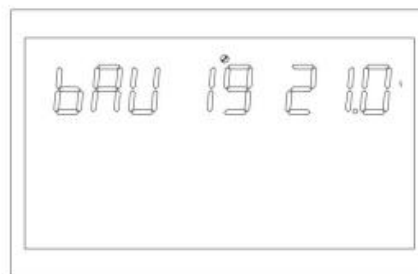
Figure 1-29 Setting the battery shutdown point
