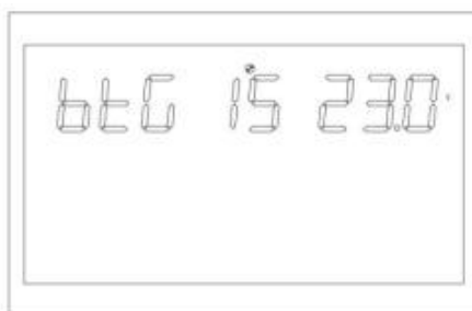
Figure 1-26 Switching the battery back to the grid voltage point
