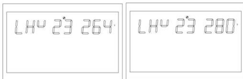
Figure 1-33 Setting high voltage point of grid
