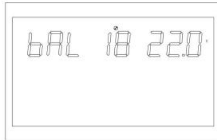
Figure 1-29 Setting the battery low voltage point
