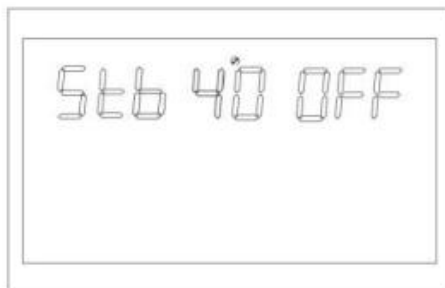
Figure 1-48 Set the SOC to turn to battery mode
