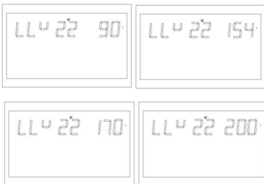
Figure 1-32 Setting the low-voltage point of grid in inverter mode
