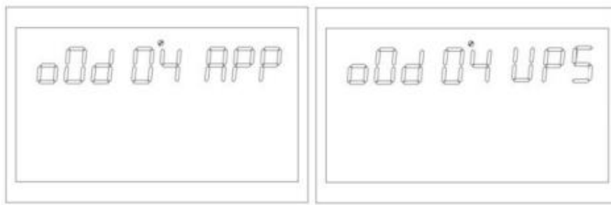
Figure 1-15 Setting the output mode
