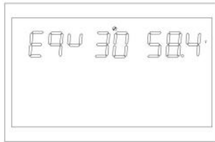
Figure 1-38 Setting the voltage balancing point
