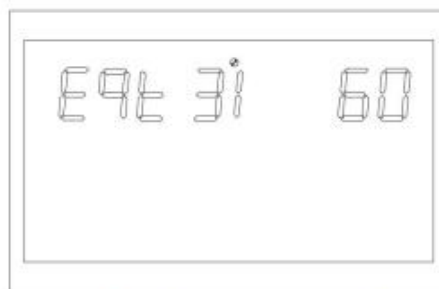
Figure 1-39 Setting the balanced charging time
