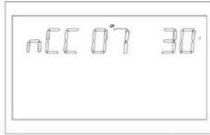
Figure 1-18 Setting the maximum charging current
