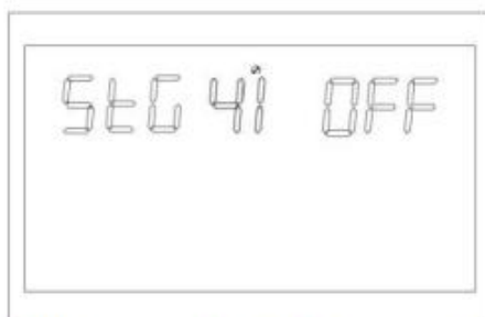
Figure 1-49 Set SOC to grid function setting page
