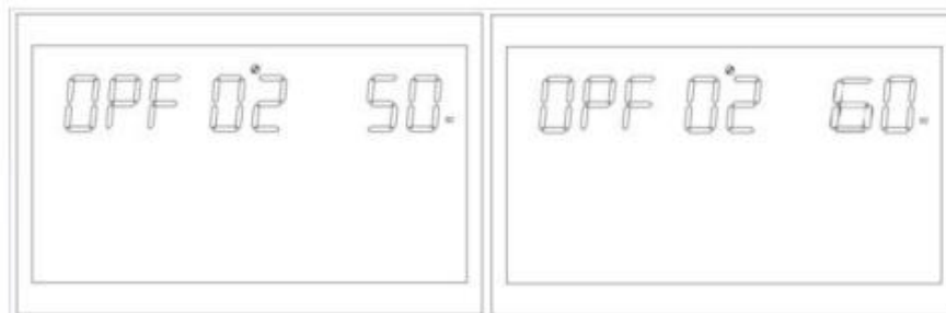
Figure 1-13 Setting the output frequency
