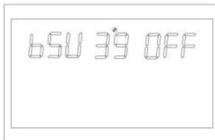
Figure 1-47 Low SOC Shutdown function setting page
